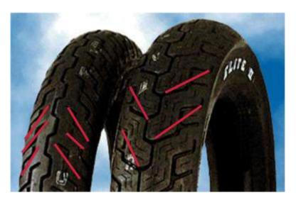
However, if you look at the front tire tread pattern of the new Dunlop Elite II's (K491) they are aligned in exactly the opposite way. That is, they tend to channel water towards the center of the tire. This CANNOT be the most effective way to diminish the odds of hydroplaning! Either the K177 or the K491 is safer on wet
