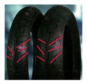
If you look at the tire tread pattern you will also see that the grooves are cut in such a way as to tend to channel water away from the center of the tire if it is rotating in accord with the arrow stamped on the side of the tire. This seems to be consistent with what the Dunlop factory rep advised in his latest message to me on the subject.
