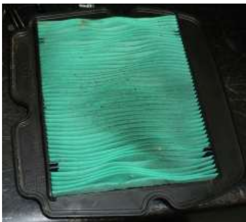
A dirty air filter - which should be changed every 12,000 miles
