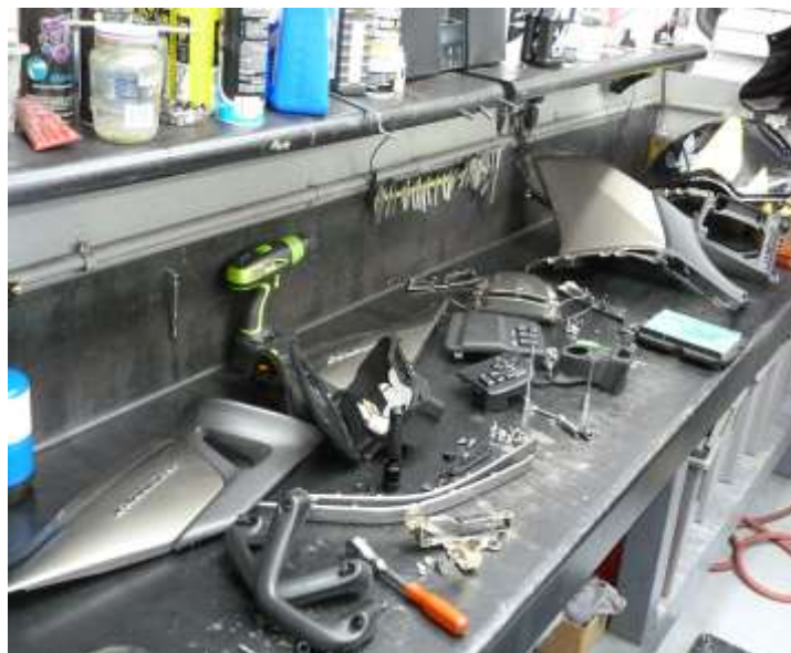
All these parts had to come off in order to get to the air filter
