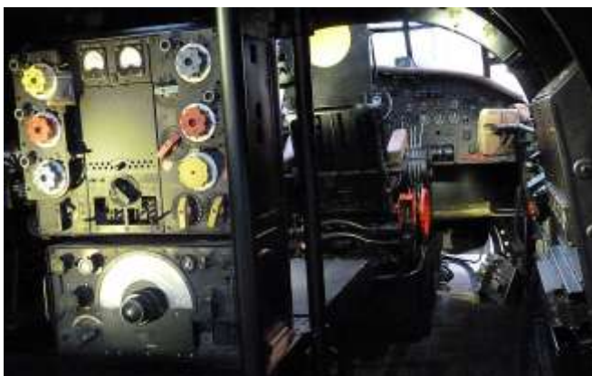
Inside view of a British Lancaster bomber—note that there is only seating for one pilot (most other bombers used two pilots)
